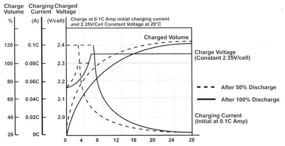
Typical characteristics for standby service type charge. Here, charging is continuous and the peak charge voltage must be lower.
