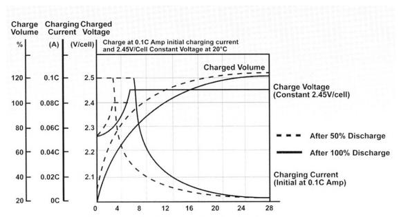
Typical charge characteristics for cycle service where charging is non-continuous and peak voltage can be higher
